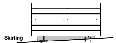
A floating skirt, powder coated in black, hides adjustable legs on inclined surfaces.
