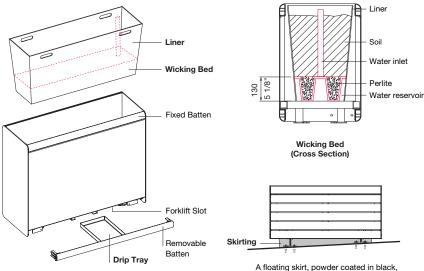
A floating skirt, powder coated in black, hides adjustable legs on inclined surfaces.
