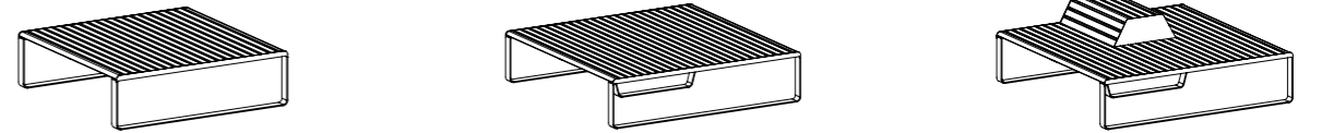
Compact size (1430mm) 1430W x 1430L x 430H mm 56 1/4" W x 56 1/4" H x 16 7/8" L Standard size (1800mm) 1800W x 1800L x 430H mm 70 7/8" W x 70 7/8" H x 16 7/8" L Standard size with Hill (1800mm) 1800W x 1800L x 650H mm 70 7/8" W x 70 7/8" H x 25 5/8" L
