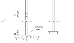
SIDE VIEW BASEPLATE CORE DRILLED SIDE VIEW BASEPLATE SUBSURFACE FIXED
